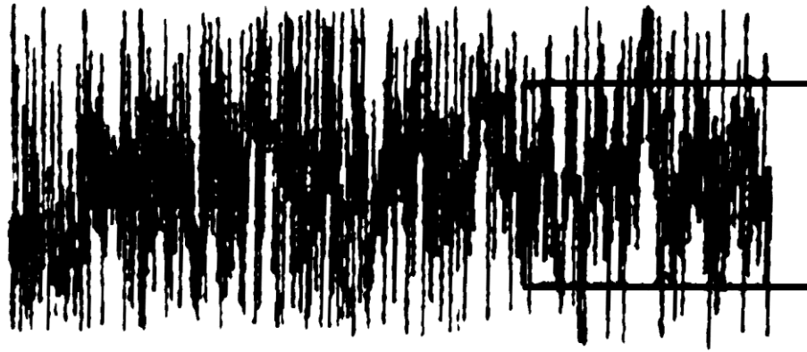
Figure 28. Scheme of EMG summary amplitude estimation. Horizontal lines run on peaks of most frequent amplitudes; vertical line is summary amplitude.
