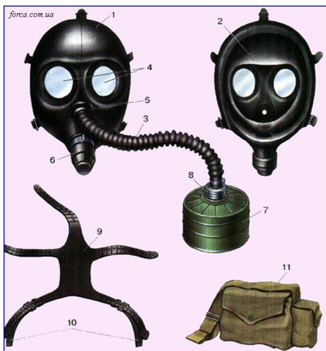
Fig. 11. Gas mask for children filtering type two, preschool for children from 1.5 to 7 years.
