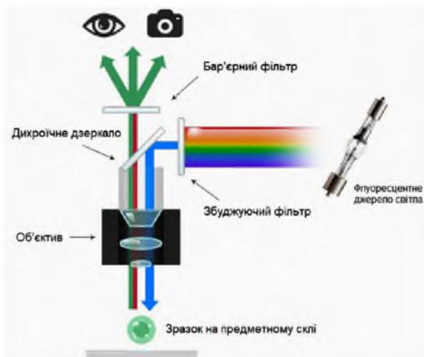
Figure 3 - Schematic structure of a fluorescent microscope
