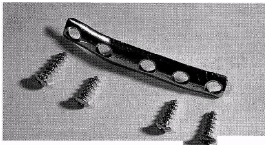
Figure 90. A standard non-compression orthopaedic plate which was removed from a treated fracture of the angle of the mandible. Insertion and removal required a large extra-oral submandibular incision.
